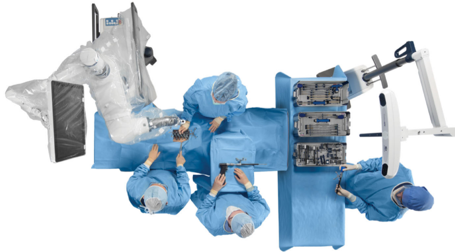
Fig. 2 Overhead schematic showing positioning and workflow with the Globus ExcelsiusGPS ® robot. (Copyright permission obtained from Globus Medical.)
