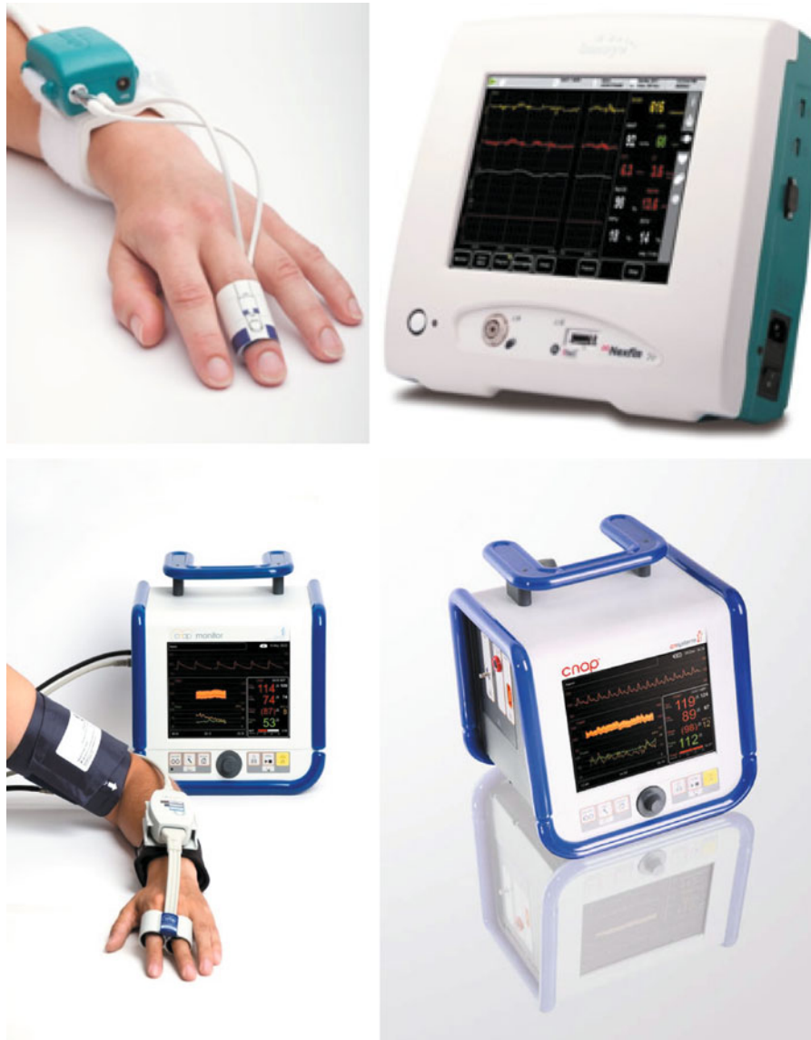
Fig. 7 Demonstration of non-invasive and beat-to-beat arterial pressure monitoring systems (“Nexfin,” BMeye [top], and “CNAP,” CNSystem [bottom]).
