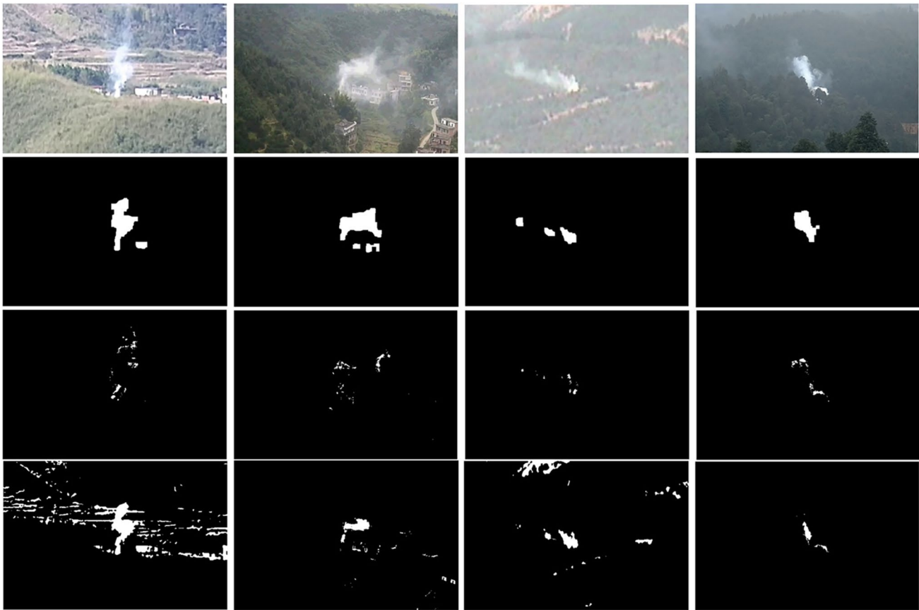
Fig. 7 Comparison between the original images (first row), the fusion images from the developed method in this study (second row), from the ViBe algorithm (third row), and from the Choquet algorithm (fourth row) for T1, T5, T6, T11
