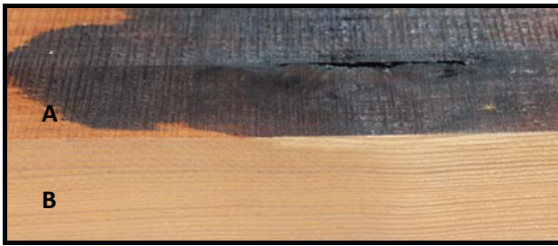
Figure 3. Release of resin on the wood surface during thermal treatment. A. Wood surface with released resin from a resin pocket before sanding, B. The same wood surface after sanding
