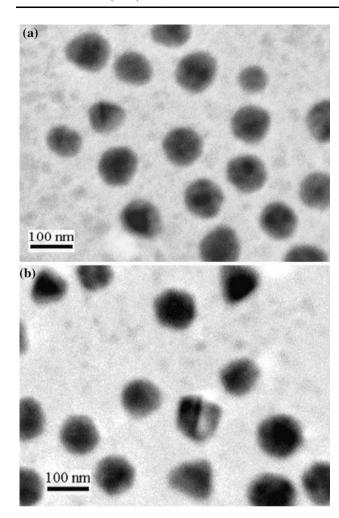
Fig. 2 TEM images of PPy/Ag nanocomposites prepared at  $[AgNO_3]/[pyrrole]$  of 0.2 (a) and 0.5 (b)
