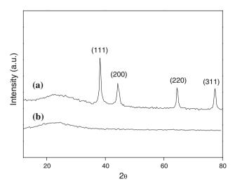
**Fig. 5** XRD patterns of PPy/Ag nanocomposite prepared at [AgNO<sub>3</sub>]/[pyrrole] of 0.8 (**a**) and PPy (**b**)
