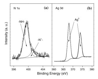
**Fig. 4** XPS N 1s (**a**) and Ag 3d (**b**) core-level spectra of PPy/Ag nanocomposite prepared at [AgNO<sub>3</sub>]/[pyrrole] of 0.8
