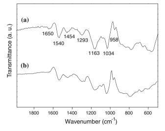
**Fig. 3** FTIR spectra of PPy/Ag nanocomposite prepared at [AgNO<sub>3</sub>]/ [pyrrole] of 0.8 (**a**) and PPy (**b**)
