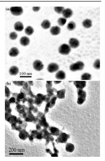
**Fig. 1** TEM images of PPy/Ag nanocomposites prepared at [AgNO<sub>3</sub>]/[pyrrole] of 0.8 with (**a**) and without (**b**) of PVP
