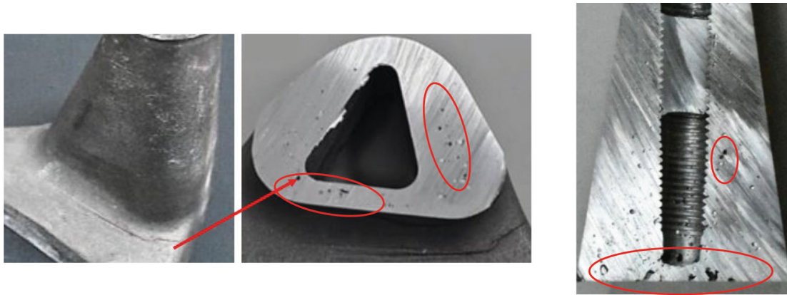
Fig. 2 Failed part cut-section images to check the porosity regions
