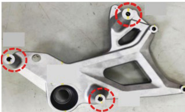
Fig. 15 Modified design swing arm—No crack confirmed through dye penetration
