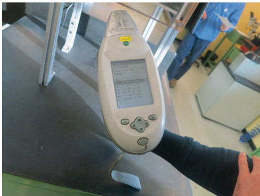
Fig. 1 A PMI device is used to determine the chemical composition of a valve body
