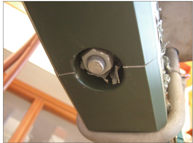
Fig. 25 Bottom view of the top saddle [15]. Reprinted from Mariusz Staco et.al, Failure Analysis of a Damaged U-Bolt Top Plate in a Leaf Spring, Proceedings of the 14th International Scientific Conference, Pages 736-743, 2019, Springer Nature
