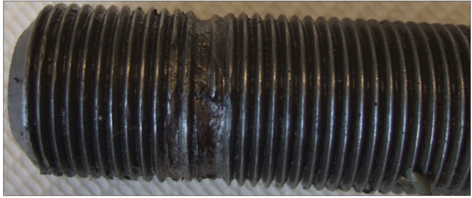
Fig. 26 U-bolt thread damage [15]. Reprinted from Mariusz Staco et.al, Failure Analysis of a Damaged U-Bolt Top Plate in a Leaf Spring, Proceedings of the 14th International Scientific Conference, Pages 736-743, 2019, Springer Nature
