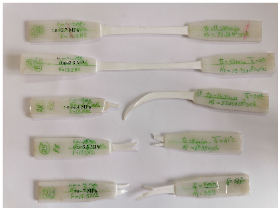
Fig. 4 Tensile fatigue test specimen stress distribution
