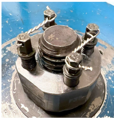
Fig. 14 Assembled jack bolt nut with jack bolt lock wire and nut body adhesive
