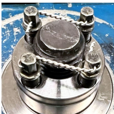
Fig. 3 Assembled jack bolt nut with lock wire on jack bolts
