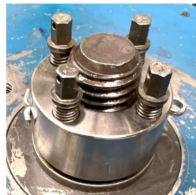
Fig. 4 Assembled jack bolt nut with cotter pin through nut body and bolt
