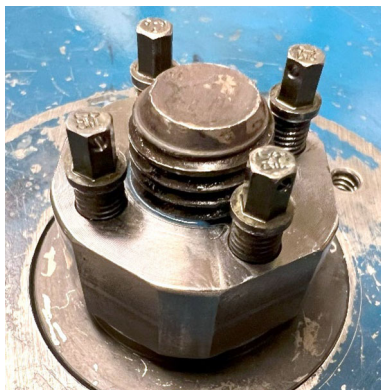
Fig. 5 Assembled jack bolt nut with added nut body wrench flats for removal with threadlocker
