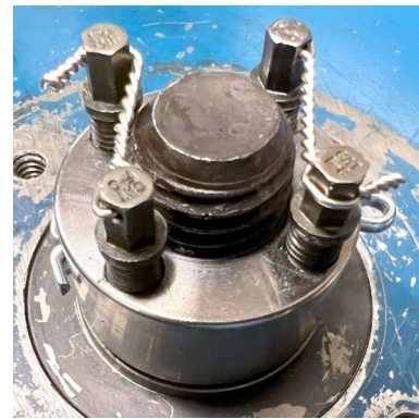
Fig. 12 Assembled jack bolt nut with jack bolt lock wire and nut body pin
