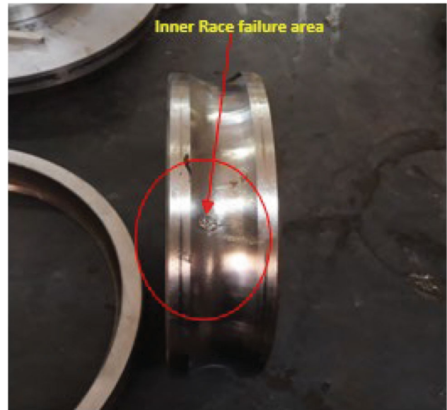
Fig. 6 Failed antifriction ball bearing
