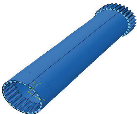
Fig. 1 Schematic diagram of transmission shaft and interior spline
