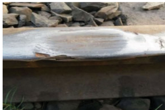
Fig. 18 Wheel burns defect [34]
