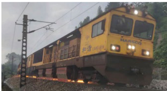
Fig. 23 Rail grinding train on the rail surface [36]
