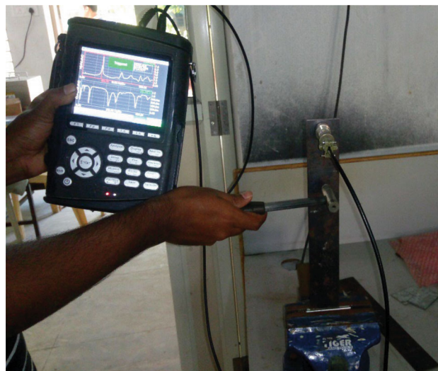
Fig. 3 Image of an impact hammer test on no cracked steel beam
