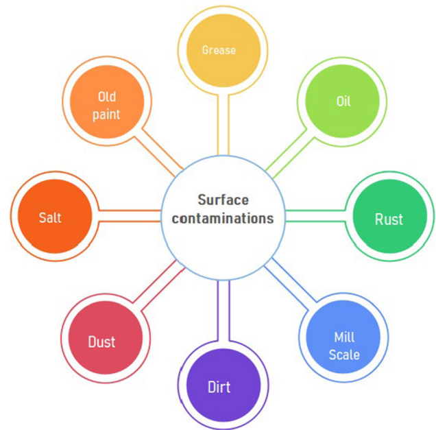
Fig. 4 Metal surface contaminants in a chart (photograph by author)
