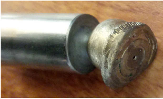
Fig. 2 The failure of the slipper pair
