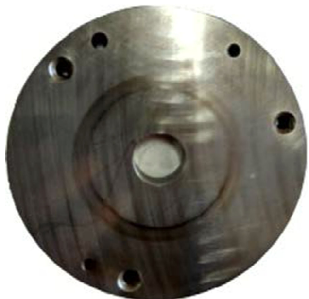
Fig. 9 The wear map of test disc
