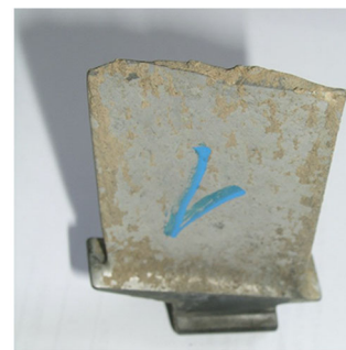
(a) Photograph of the portion of the fractured blade that remained attached to the rotor.
