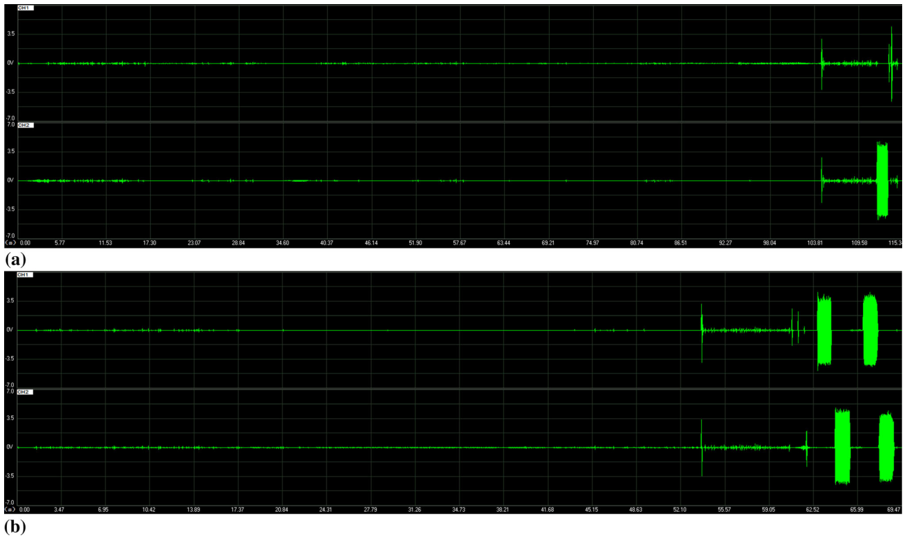
Fig. 4 Time (unit: s) versus amplitude (unit: V) for AE waveforms during fatigue tests for a specimen-1 and b specimen-2
