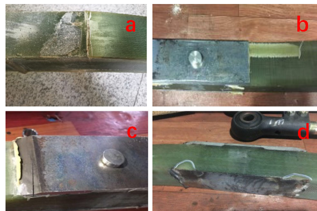
Fig. 10 Failure picture of the middle of the leaf spring
