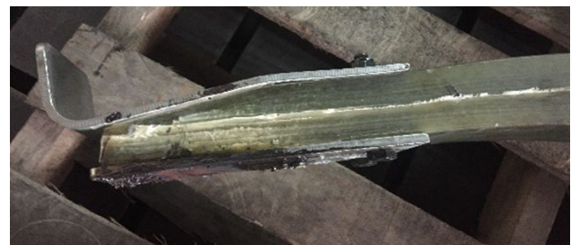
Fig. 14 Failure of the leaf spring end
