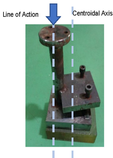
Fig. 6 Eccentric load at fixture
