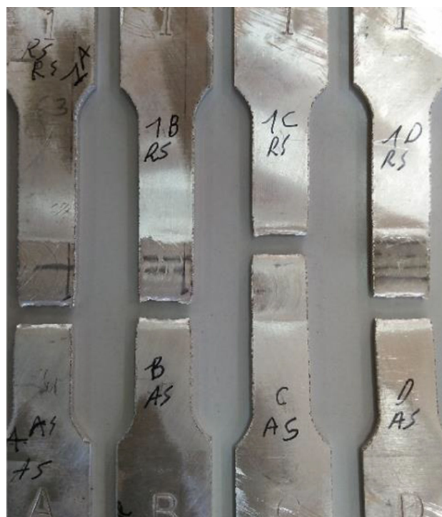
Fig. 8 Tensile specimen after test
