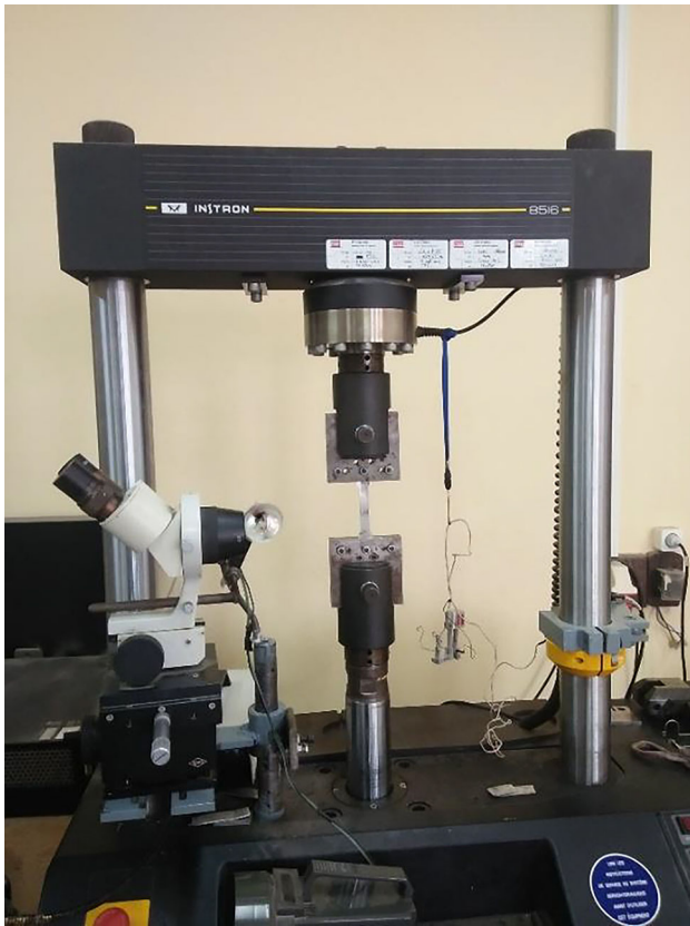
Fig. 3 Universal machine used for tensile tests
