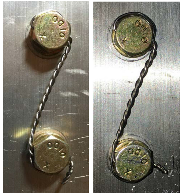
Fig. 2 Safety wired bolts using double twist method: Inconel and stainless steel
