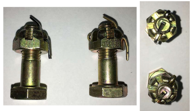
Fig. 5 Castellated nut, cotter pin and bolt assemblies using preferred method
