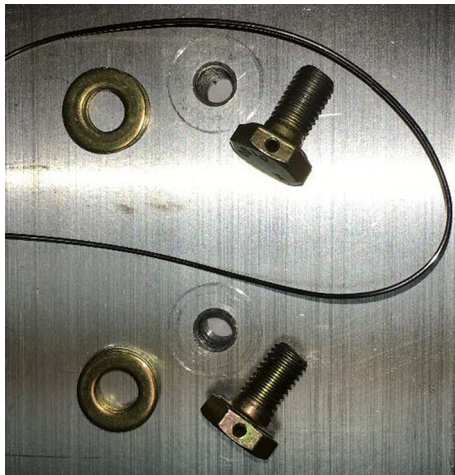
Fig. 1 AN bolts with washers, aluminum plate and safety lock wire
