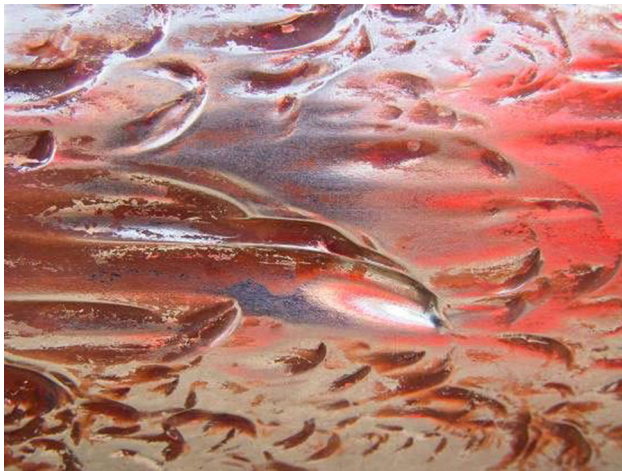
Fig. 1 Macro-damage morphology of downhole tubular outer surface caused by erosion–corrosion
