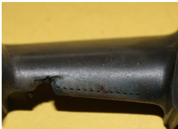
Fig. 4 Metal chip-off in HP turbine rotor blade
