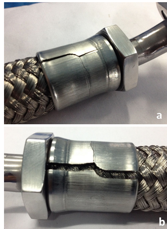
Fig. 3 Digital photograph showing the cracking of sleeve in hydraulic pressure set-up (a) and after removal from the set-up (b)
