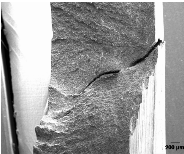
Fig. 6 SEM image showing a full view of the fracture surface through the complete thickness of the sleeve
