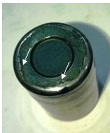
Fig. 4 Material flow observed on roller head (shown by arrow)
