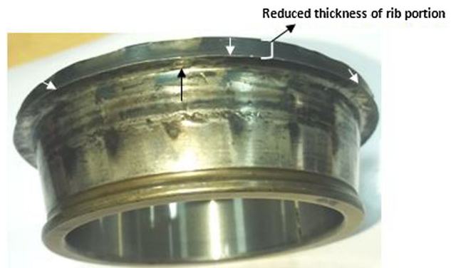
Fig. 3 Cone component in as-received condition; wedge-shaped protrusion on rib portion is shown by white arrows; black arrow points to the plastic flow in the groove portion
