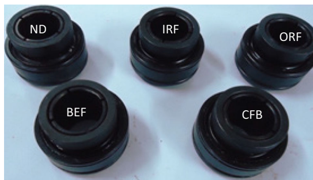
Fig. 4 Rolling bearings with five individual fault conditions
