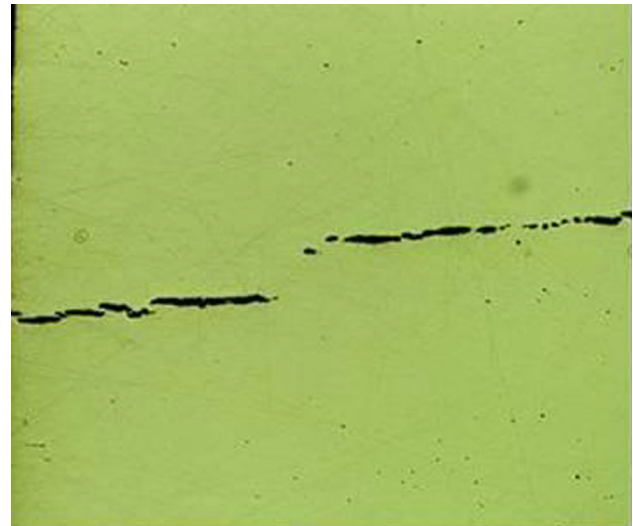
Fig. 4 HIC in the SWC form, Mag. \times 40 , unetched
