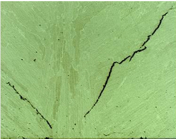
Fig. 5 SSC in the weld seam, Mag. \times 20
