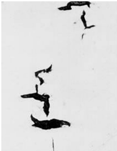
Fig. 3 SOHIC at the tip of one crack showing stacking of cracks perpendicular to the applied stress. As polished, Mag. \times 50
