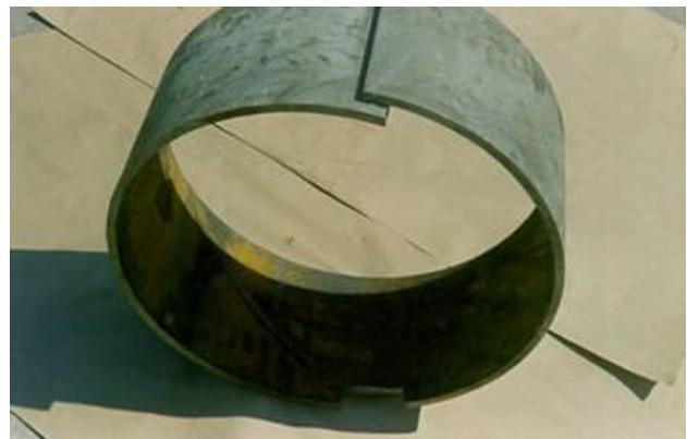
Fig. 1 Ring cut from failed spiral pipe showing compressive macroscopic residual stress
