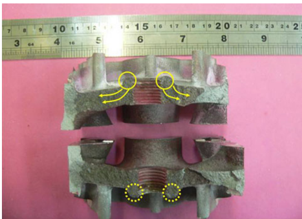
Fig. 6 The surfaces after opening cracked zone
