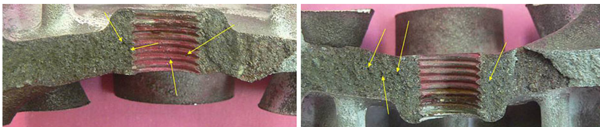
Fig. 7 Pores around the hole due to the casting process
