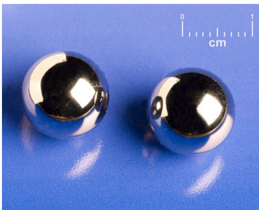
Bearing balls made from 60NiTi. They are highly corrosion resistant and resist denting because they are within the rare class of “superelastic” materials
