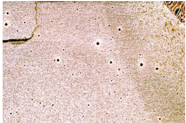
Fig. 4 HIC located outside the heat-affected zone in specimen no. 7-W-A, heat no. E, Mag. 32×
