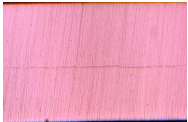
Fig. 5 HIC due to centerline segregation in specimen U-B, Heat No. G
