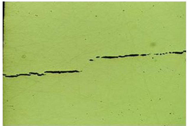
Fig. 7 Stepwise cracking in Pipe No. D0307882, Heat No. V, Mag. 40×
