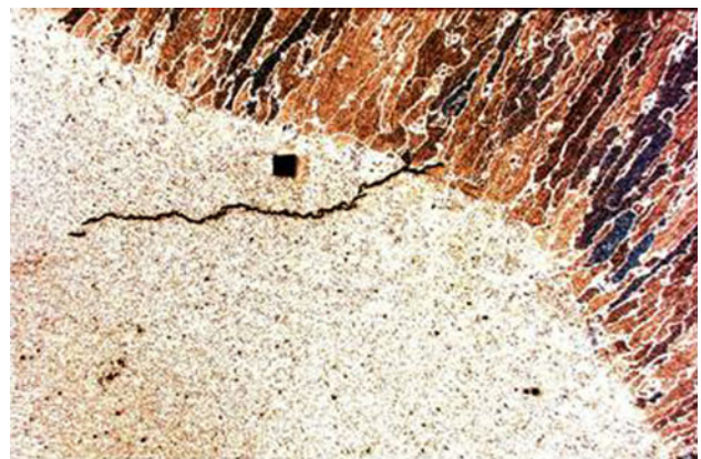
Fig. 8 SSC in the HAZ terminating at the vicinity of the fusion line. Pipe No. D0307143, Heat No. X, Mag. 16×
