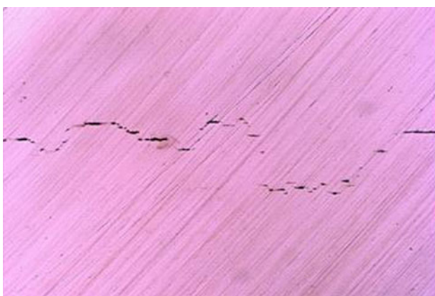
Fig. 3 Stepwise cracking in Pipe No. 5, heat no. B, Mag. 20×
