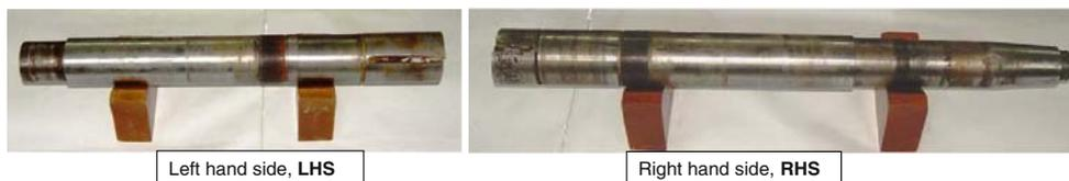
**Fig. 3** Fractured surfaces before cleaning showing final fracture opposite to key slot
