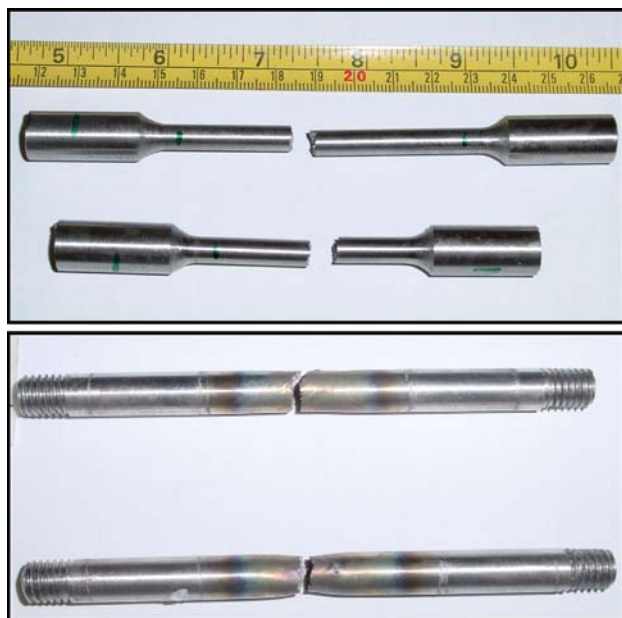
Fig. 10 Tensile samples at room temperature (RT-top) and at 800 °C after the test. The samples of the RT show no plastic deformation, indicative of brittle fracture; while slight necking is observed in the high-temperature tests
