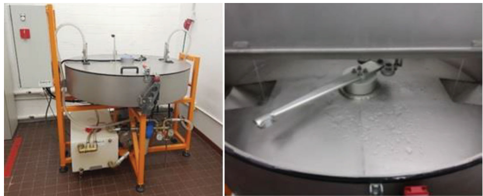
Fig. 5 Jet erosion equipment (a) and central rotating arm (b)
