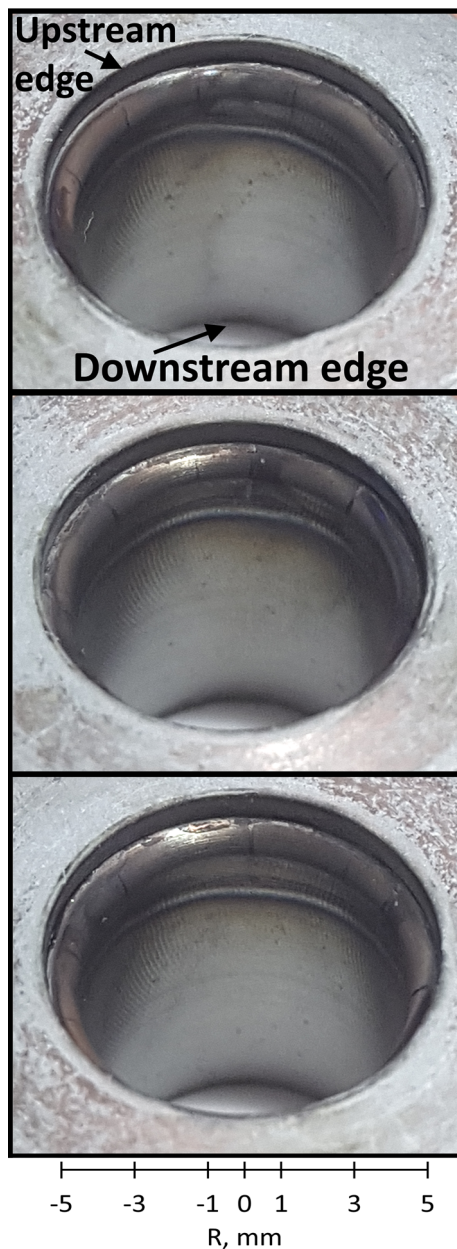
Fig. 14 Photographs of SinplexPro new anodes tested for 5 min with 500 A and 60 NLPM of argon from three different angles. The whole circumference is shown
