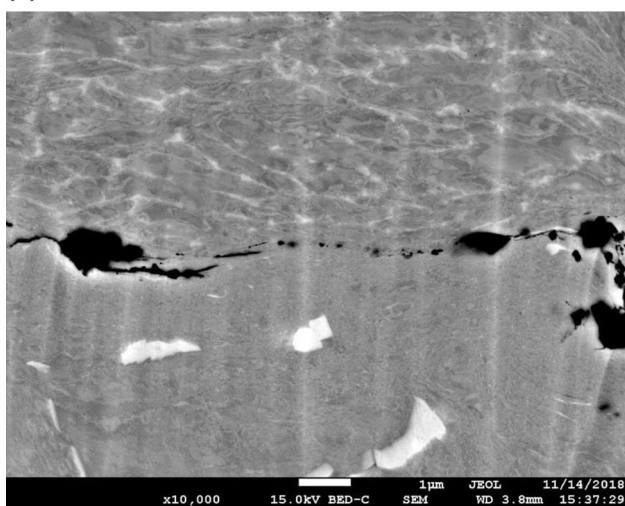
Fig. 11 SEM micrographs of the interface region of coating (top) and substrate (bottom), left as-sprayed, right annealed conditions (500 °C, 1 h). The dark lines are cracks, the larger black areas are remainings from the grit blasting process ( \text{Al}_2\text{O}_3 ), and smaller spherical features are pores
