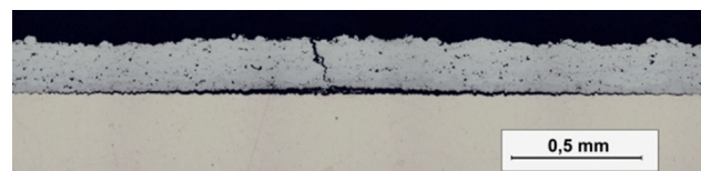
Fig. 15 Cross section of a coating which buckled during laser cycling. Coating thickness: 180 \mu\text{m} , surface temperature: 1118 K
