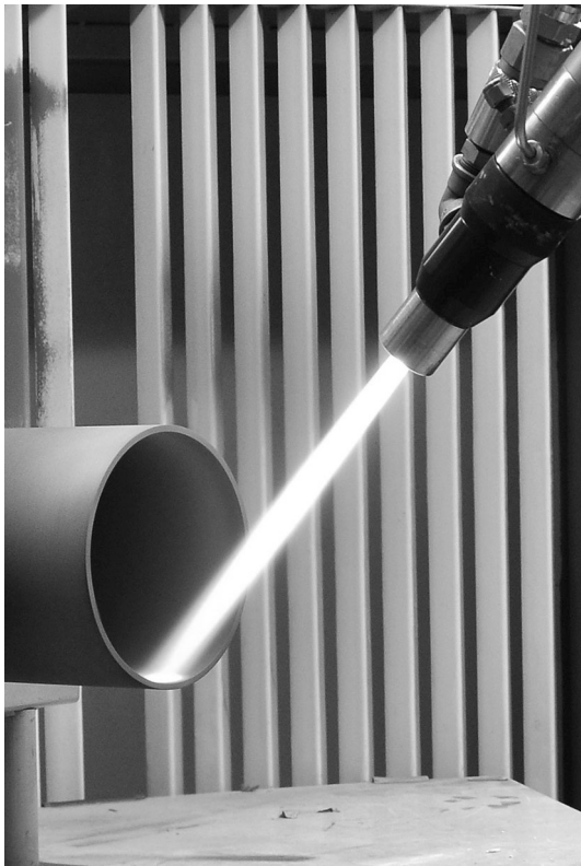
Fig. 1 Off-angle spraying of a tube (internal diameter 160 mm)
