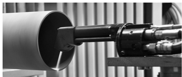
Fig. 2 IDCoolFlow Mono; ID spraying of a tube (internal diameter 160 mm)
