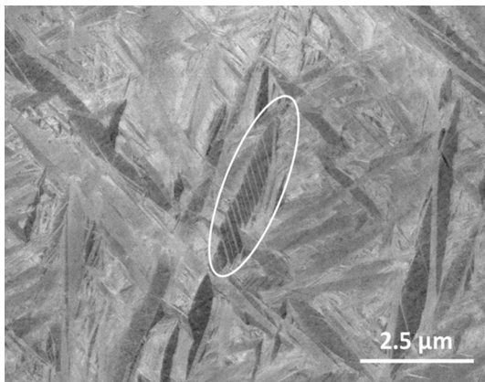
Fig. 4 ECCI of the powder cross section of spherical Ti6Al4V powder showing dislocation twins inside the martensitic laths (features inside the white oval)
