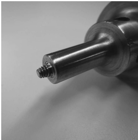
Fig. 6 FSW Tool fabricated from H13 tool steel with a MP159 pin
