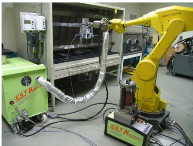
Fig. 4 CGT 4000 high-pressure cold spray system used to produce the transitional layer
