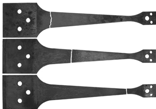
Fig. 5 Fractured corrosion fatigue test specimens of bare X80 steel under 333 MPa
