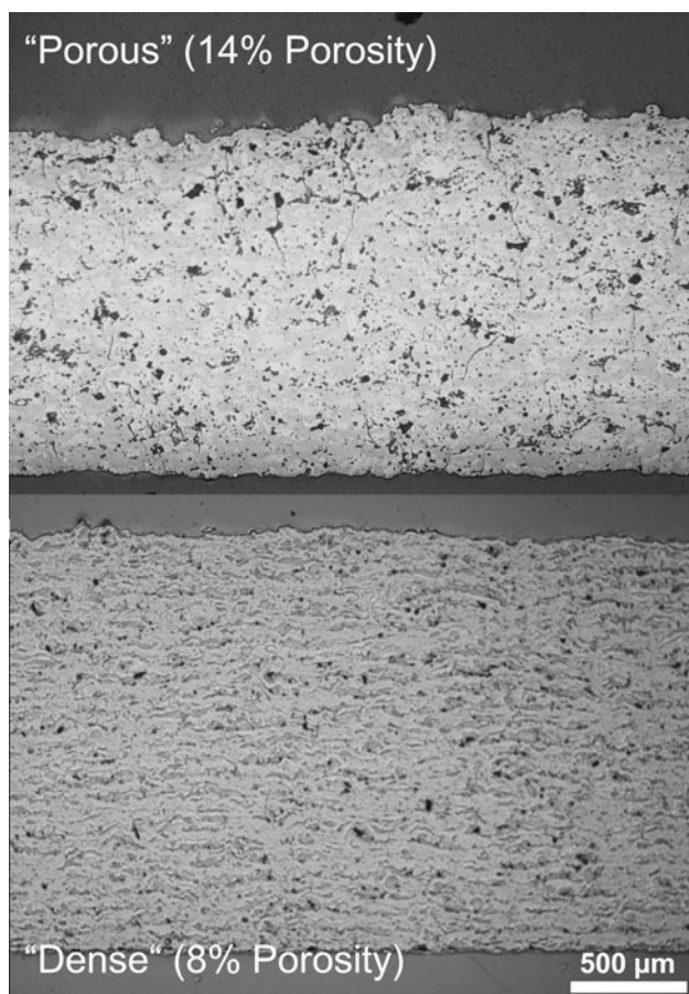
Fig. 10 Optical micrographs of \text{LaLiAl}_{11}\text{O}_{18.5} hexaaluminate coatings manufactured with parameters as summarized in Table 1
