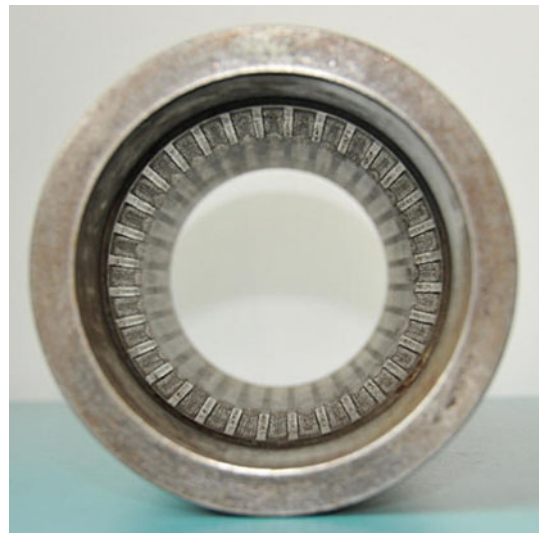
Fig. 6 A short rifled gun barrel for push testing
