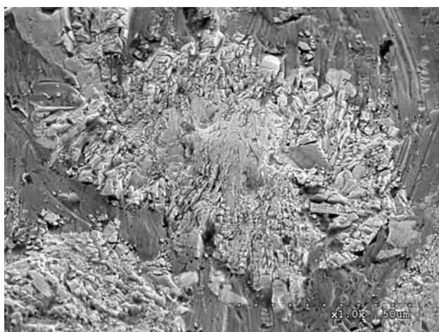
Fig. 7 SEM micrograph showing the surface of the 6040 overlay, after abrasion by the 20/30 mesh sand. Magnification 1000×
