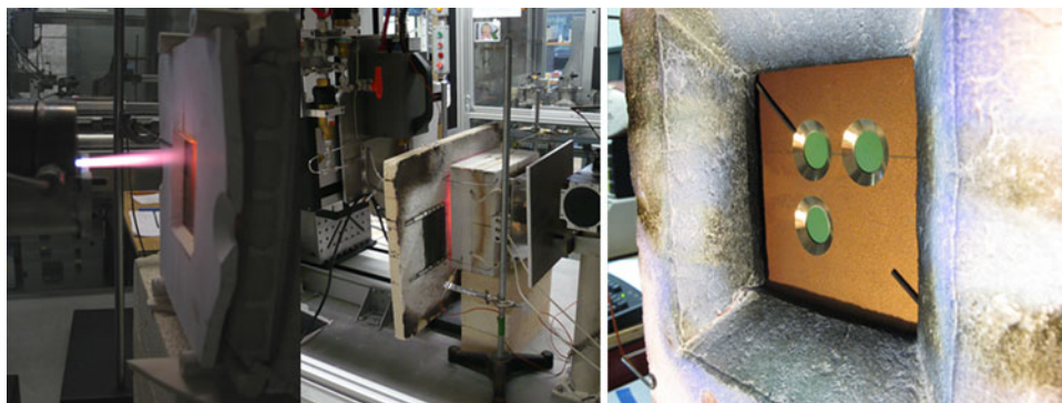
Fig. 3 Reactive Spray Deposition Setting for SOFC deposition on anode supported cell showing in order the front side deposition, back side heating block and circular mask for deposition
