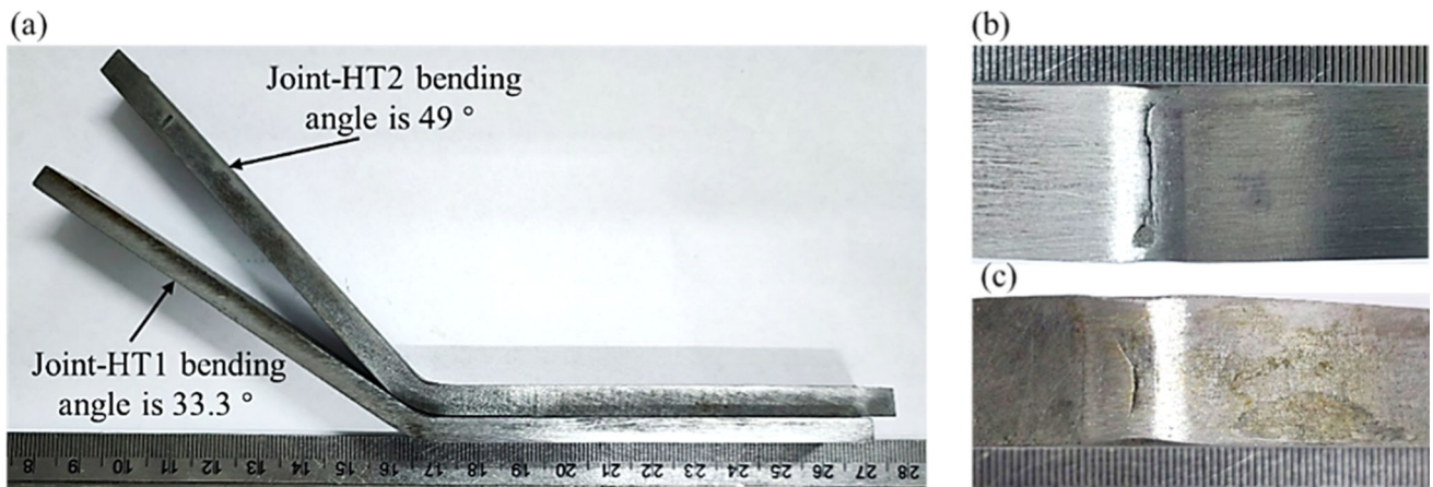
Fig. 17 Three-point bending test results of two quenched and tempered welded joints at room temperature
