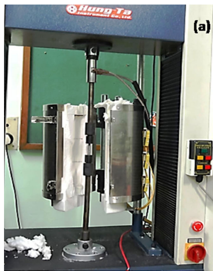
Fig. 2 Tensile testing of SS321: (a) HungTa tensile testing machine and (b) schematic of the tensile specimen (dimensions in mm)
