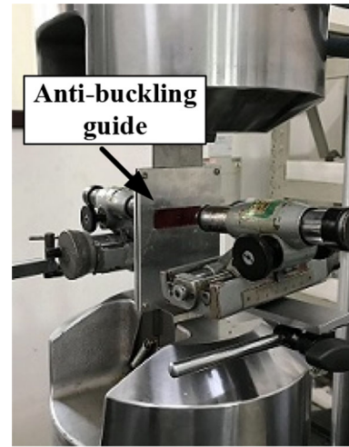
Fig. 4 Fatigue crack growth test
