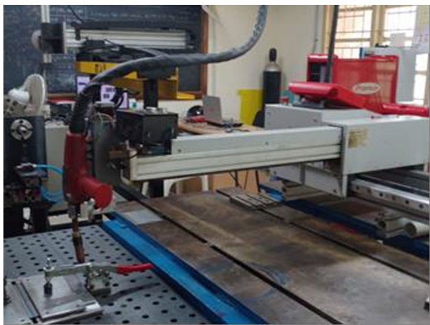
Fig. 1 Photographic view of cold metal transfer machine
