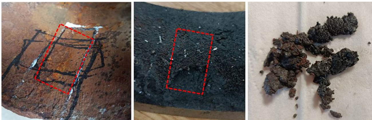
Fig. 2 L245NS and L360QS steel and inner pipe wall attached with gum. (a) L245NS steel (b) L360QS steel (c) gum
